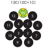
Figures in  $\bigcirc$  indicate white numbering on black insulator.
