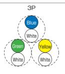
The first core is white insulator, the second core is blue insulator. Moreover, numbering the pair number.
