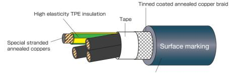
Low friction, oil, heat, flame resistant and flexible PVC sheath(Dark Blue)
