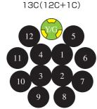
Figures in  $\bigcirc$  indicate white numbering on black insulator.
