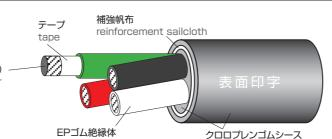
※12心以上はより合わせ上にテープ巻き/Cables with more than 12 cores: binder tape on cores.
